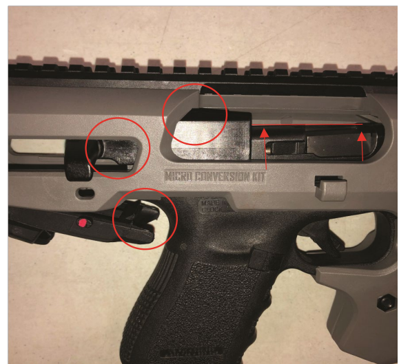
Figure 3B: Rear sight improperly installed.
